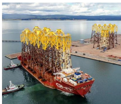
Fondations jacket (stockage et transport)
