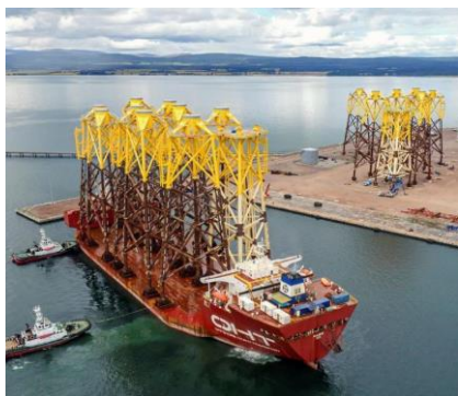
Fondations jacket (stockage et transport)
